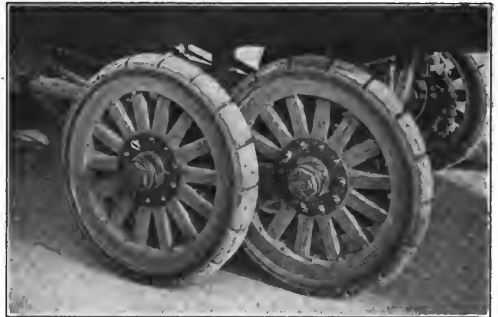
Fig. 3—Dow wheels have minimum clearance
